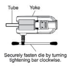
4) Grasp the yoke and rotate the hydraulic cylinder clockwise until it stops.
