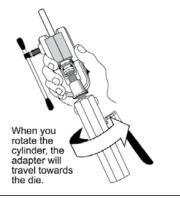
Begin squeezing the lever and continue until the edge of the adapter meets the die or pumping action shows substantial resistance.
