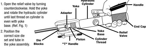
Tube end should be even with face of die blocks for swage and even with mark on die blocks for flare. (Ref. Fig. 2)
