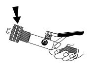
De-burr the inner walls of the tubing completely and make sure the tube will fit easily over the expander head.
