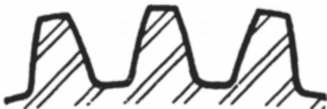
4 Diametral Pitch .7854" Circular Pitch
