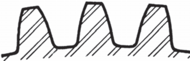
3 Diametral Pitch 1.0472" Circular Pitch
