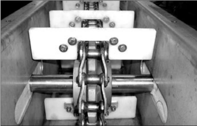
Welded Steel Chain and Sprocket
