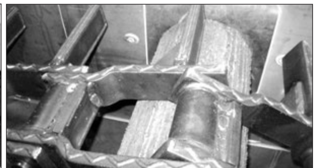
Special Mill Duty Drag Chain - Flight and Idler
