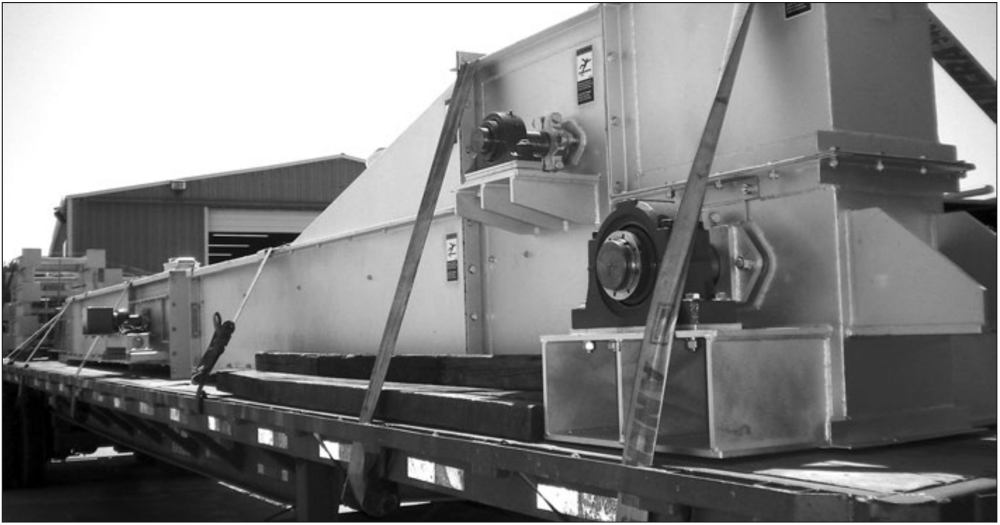
MSC Super Capacity Drag Head with Slack Side Tension Idler Sprocket
