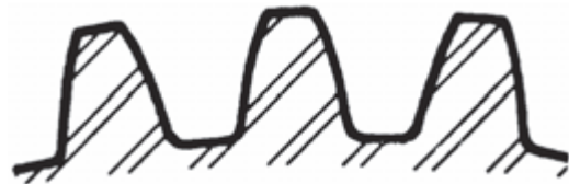
3½ Diametral Pitch .8976" Circular Pitch
