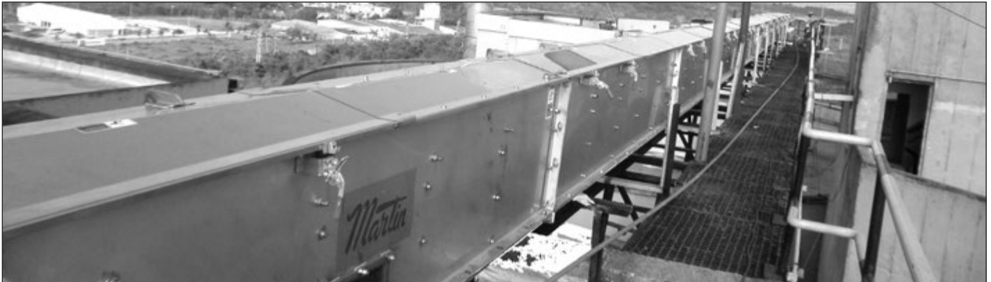
Field assembly of Martin MFB™ Drag
