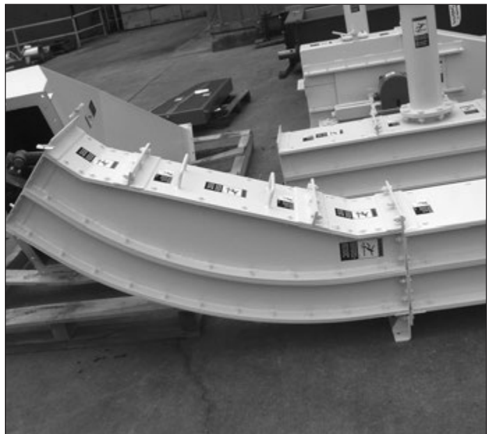
MMD Special L-Path Drag with Slack Accommodating Bend
