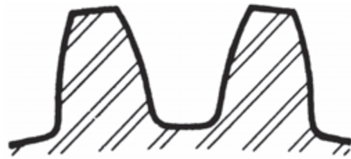
2½ Diametral Pitch 1.2566" Circular Pitch
