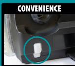
Oil level visible through large window for easy sight check of bar lubricant
