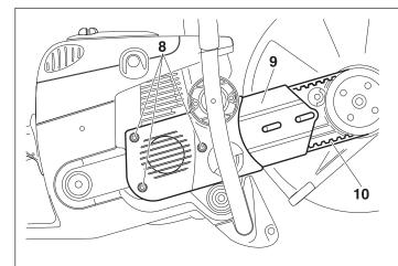
Unscrew the screws (8) and remove the crankcase housing cover (9).
