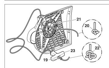
Thread in a new starter cable (dia 4.0 mm, length 1000 mm) as shown (don't forget the disc (19)) and knot both ends.
