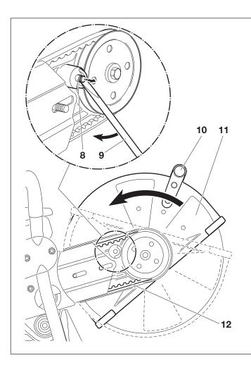
Use the combination tool (8) to lever out the stop pin (9) as shown in the illustration, until the protective hood (11) can be turned.
