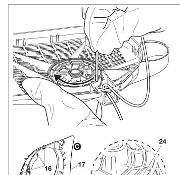
Guide the cable into the recess (24) on the cable drum and use the cable to turn the drum two turns in the direction shown by the arrow.
