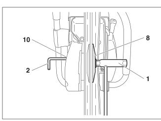
Place the spring washer (8) on the arbour and insert the screw (9) and tighten by hand.
