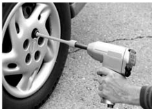
Torque Extensions used with your 1/2" drive impact wrench and lug nut sockets
