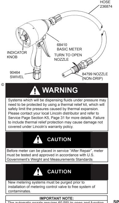
The automatic nozzle requires 60 PSI to open and function properly. A pump exceeding 60 psi is required for adequate flow and proper operation. A pump ratio of at least 3:1 is recommended.
