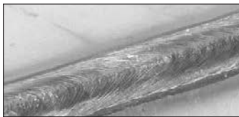
Power Mode® reduces spatter and improves bead appearance, even for low voltage procedures on stainless.
