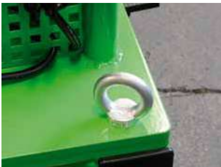
The puller can be moved by a crane using the provided mounting eyelets.
