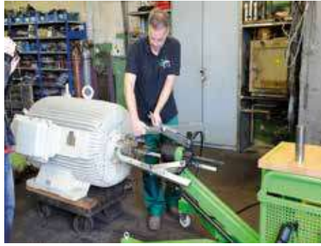
Place the pulling hooks on the part to be pulled and secure them with a wrench. Ensure that they are properly fitted and make uniform contact.
