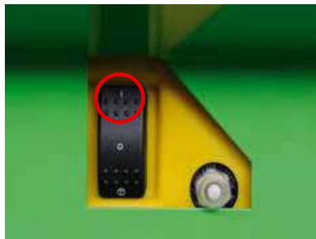
Put the power switch in the On (I) position.
