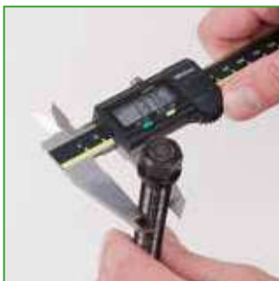
a Measure the spindle diameter.
