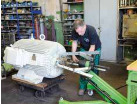
Fit the pulling hooks to the part to be pulled.
