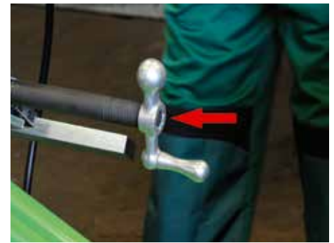
Fit the hand crank on the square end of the spindle. Then turn the crank until the spindle is centered and pretensioned hand-tight.
