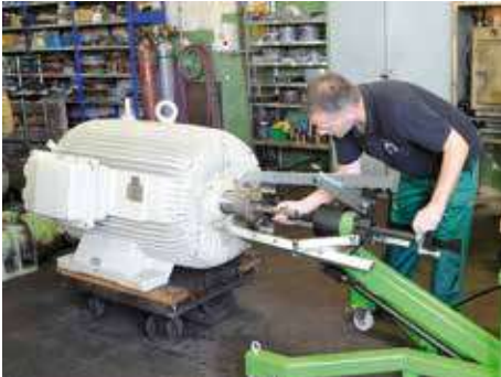
The spindle must be centered and pre-tensioned hand-tight using the hand crank.
