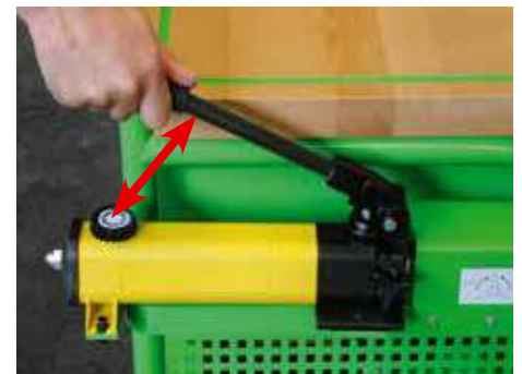
Use the hand pump to raise the puller to the necessary height.
