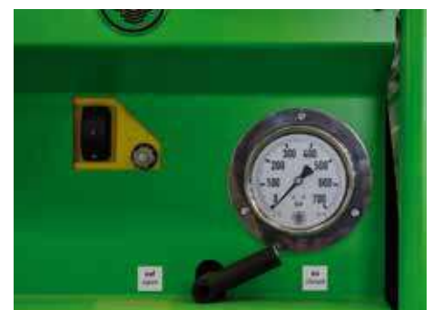
A pressure gauge can be fitted to check the applied pulling force.
