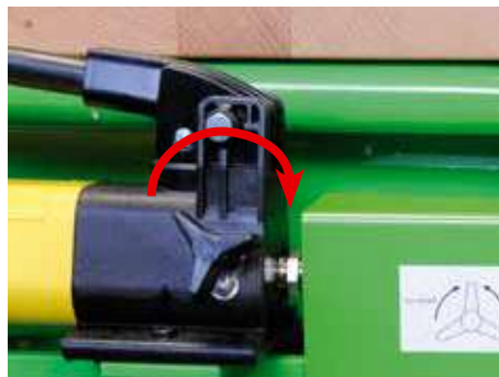
Close the shut-off valve before operating the hand pump.
