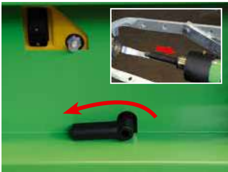
After completion of the pulling process, open the shut-off valve. The spindle retracts automatically.
