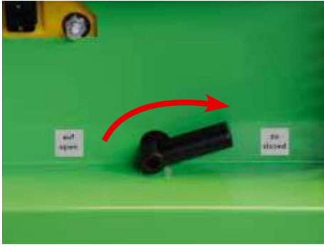
Close the shut-off valve for starting the pulling process.
