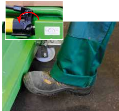
Step on the foot pedal while opening the shut-off valve of the hand pump.
