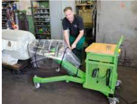
Completely surround the puller with a protective tarp (UFP-3).
