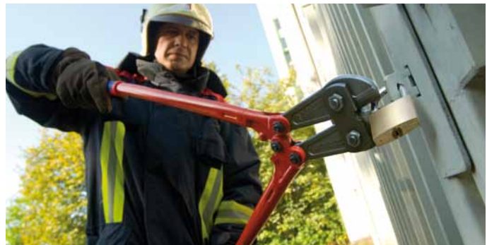
Forged-on stopper with absorbing inserts: cushions the cutting stroke
