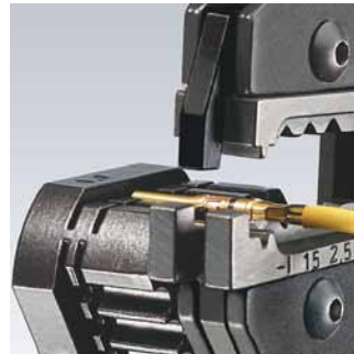
97 43 200 with crimping dies 97 49 61 and locator 97 49 90 for turned types of connectors with varying pin diameters, revolvable
