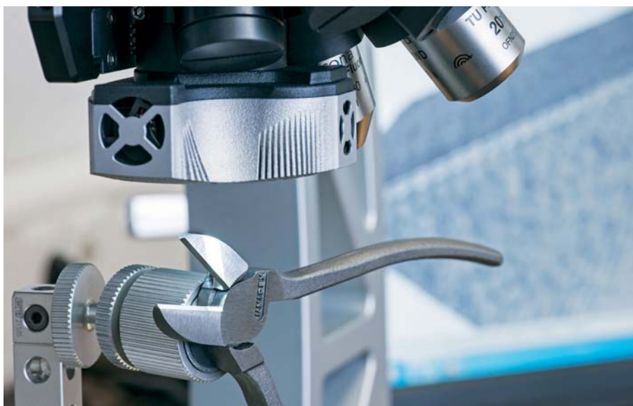
Shape and roughness of the diagonal cutter's cutting edge are precisely measured with an optical 3D measuring system.
