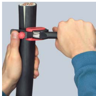
Turning the tool for circumferential cut
