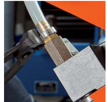
Sealing the hose connection on central lubrication
