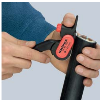
Setting the tool for longitudinal cut
