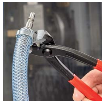
Sealing the pneumatic hose on the quick action coupling using the side press nib
