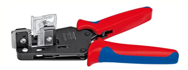
For materials such as rubber cable we recommend Precision Insulation Strippers 12 12 xx. These pliers work with two precise pairs of blades which cut through the insulation across the entire circumference of the cable. They are therefore also ideal for difficult materials such as rubber, PTFE or silicone.
