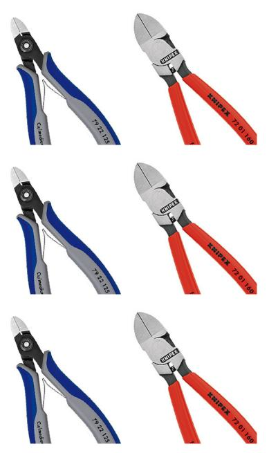
The frequently used 78 models (Electronic Super Knips®) are almost at the limit of their load-bearing capacity when cutting cable ties, especially in the case of wide cable ties or when they are cut using a fast cutting movement: the speed increases the friction.
