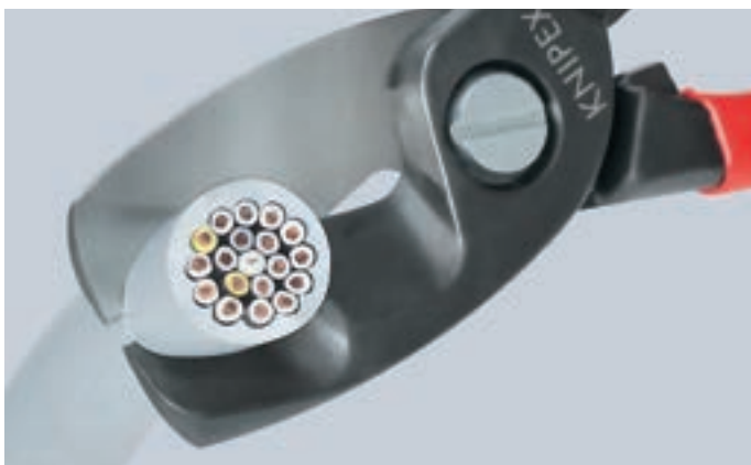
Initial cut: using the front cutting edge to cut the insulating sheath on larger cable diameters leaves an ergonomic handle opening width.
