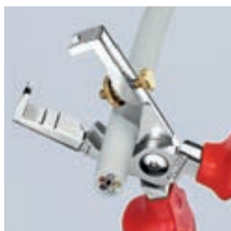
Induction hardened shear blade with precisely ground cutting edges for crushing-free cutting of copper cables up to Ø 15 mm (5 x 2.5 mm 2 )
