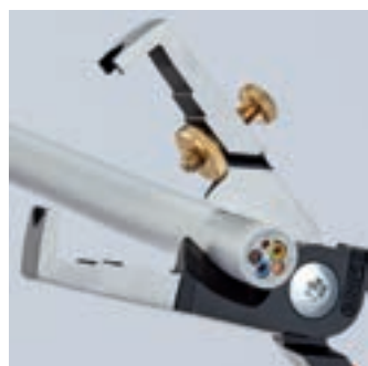
Induction-hardened shear blade with precisely ground cutting edges for crush-free cutting of copper and aluminium cables of up to Ø 15 mm (5 x 2.5 mm 2 )
