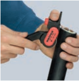
Setting the tool for longitudinal cut
