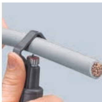
Setting the tool for circular cut
