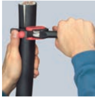
Turning the tool for circumferential cut
