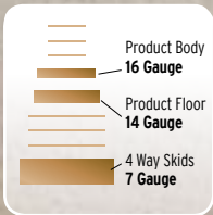
STEEL GAUGE CONSTRUCTION
