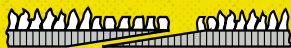
Type 2 Diagonal cut, glued overlapped. Grain tips are completely removed from the overlap to provide for a smoother running belt.
