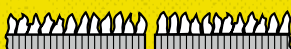
Type 3 G Zig zag joint, with cloth-reinforced foil backing, impact-free working at very sensitive parts, in particular glass.
