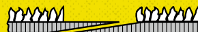
Type 5 Overlapping glued joint. Grit zone is completely ground off. Preferred joint for wood finishes with flat contact elements.
