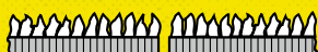
Type 4 G Diagonal cut. Butt joint with cloth-reinforced foil backing. Also suitable for working on unsupported belts, for demanding requirements.
