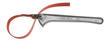
The Klein Tools 12-Inch Grip-It Strap Wrench is completely adjustable for tight-quarters tasks on polished, PVC and glass pipes, fittings, filters, conduit and shafts. The strap is urethane-coated to resist scratching or damaging surfaces and is attached to a lightweight I-beam handle. Also available in 6-Inch and 18-Inch lengths (Cat. No. S6H and S18H).
