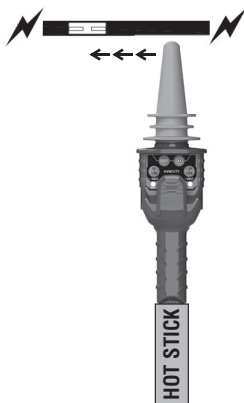
Fig. 2: Finding a cable fault
