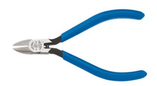
These Electronics Pliers have a tapered nose for easy working in confined areas and close tip cutting. The short jaws have beveled edges for semi-flush cutting of wire. The induction hardened cutting knives and hot-riveted joint ensure smooth action and long life.
