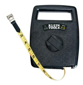
Klein Tools 50-Foot (15.24 m) Tape Measure is made from woven fiberglass tape with moisture-proof coating of polyvinyl chloride assures durability and protects against oil or chemicals. All metal parts are nickel plated for protection against rust. Tape line is graduated in feet and inches to 8ths.
