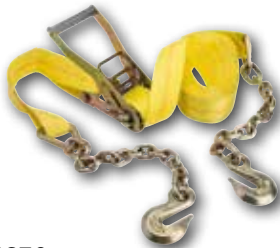
04650 27' x 2" Ratchet Tie-Down w/Chain Ends & Grab Hook 3,333 lbs. WLL 10,000 lbs. Break Strength
