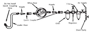
The air inlet, used for connecting air supply, has standard 1/4" NPT American Thread.
