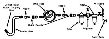
The air inlet, used for connecting air supply, has standard 1/4" NPT American Thread.
