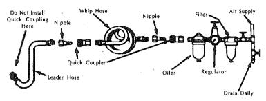
The air inlet, used for connecting air supply, has standard 1/4" NPT American thread.
