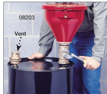
Pushing down handle opens ball valve to release liquid into drum.
