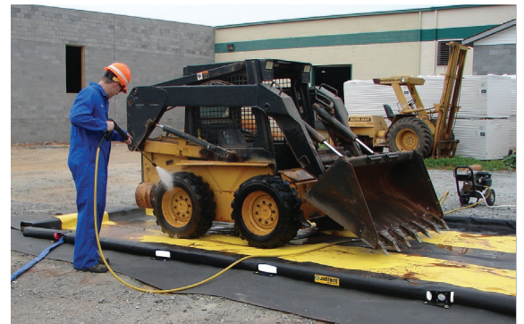
Wash down dirty equipment and recapture water for reclamation.
