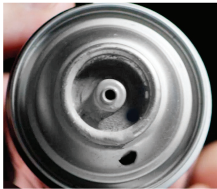
Smooth side puncture leaves no jagged edges.
