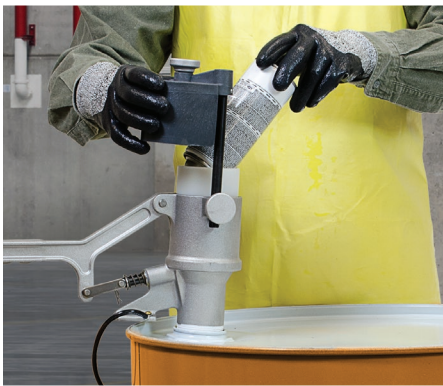
Insert inverted can into sleeve, rotate safety shield, and twist knob for secure closure to reduce spray back.
