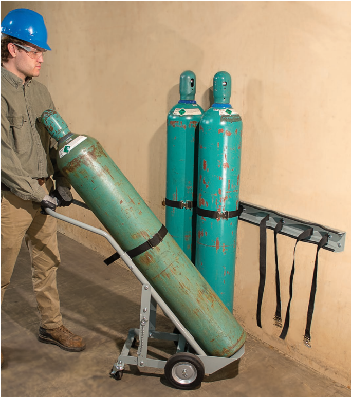
All compressed gas-cylinders in service or in storage at user locations should be secured to prevent falling or rolling.
