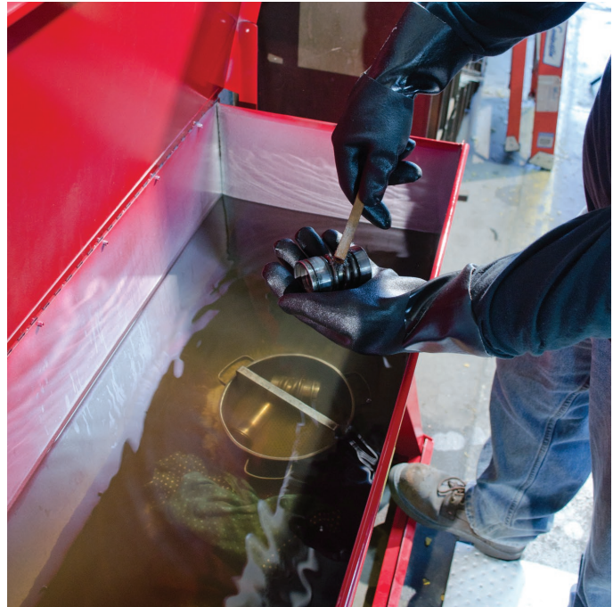
Foot treadle opens the rinse tank cover, leaving hands free for cleaning.
