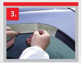
3. To mask along a straight section, tear off a section no longer than 20cm, slide in and leaver back the trim ensuring it overlaps the last piece.
