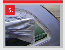
5. Allow paint to dry and remove all the masking materials.
