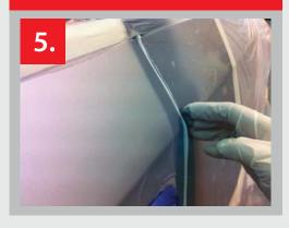
5. Adjust the material back into the gap ready for painting.
