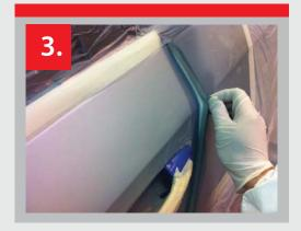
3. Prime the panel and then pull the outer piece away from the panel to expose the unprimed material below.
