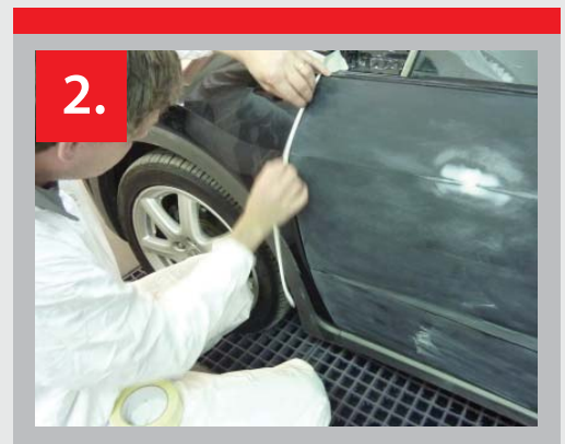
2. Apply the tape in the gap smaller side first. Locate the tape in the gap so that it sits in the central groove.
