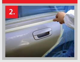
2. Apply the tape onto the panel next to the swage line ensuring that the tape edge is level with the panel bend. Then mask the rest of the vehicle.
