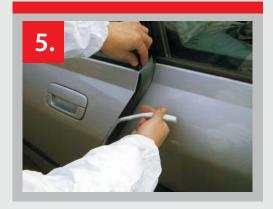
5. Once the paint is dry, remove all the masking materials.
