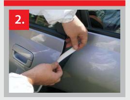
2. Apply tape behind the door edge taking care to place the adhesive behind the panel. Leave the adhesive free portion extending beyond the door edge.
