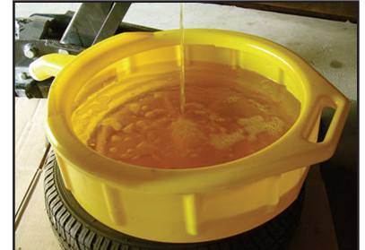
Draining gasoline into an open container is not safe or efficient and not a recommended practice.
