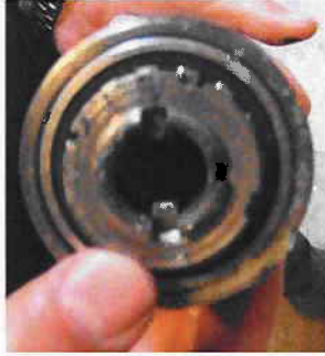
Figure 16 Nut for adjusting the play of the quill
