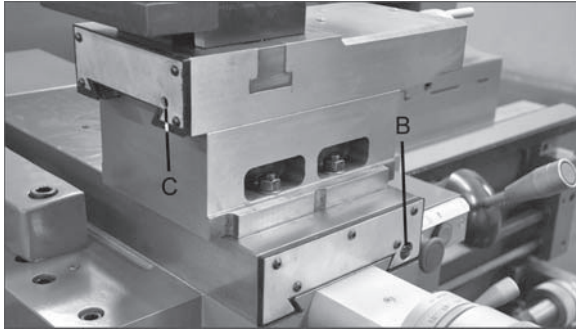
Figure 36 – Gib adjustments, slide and rest
