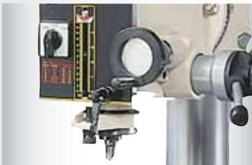
DEPTH STOP - WHEN SET THE QUILL WILL ONLY ADVANCE TO THE SET DEPTH
