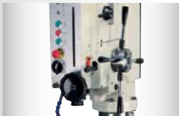
SPEED AND FEED SELECTORS ARE LOCATED ON ONE SIDE OF THE DRILL FOR EASE OF OPERATION
