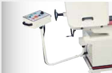
SWING AWAY CONTROL PANEL
