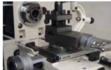
COMPLETE WITH 4-WAY TOOL POST AND 3-JAW CHUCK MOUNTED FOR EASE OF USE
