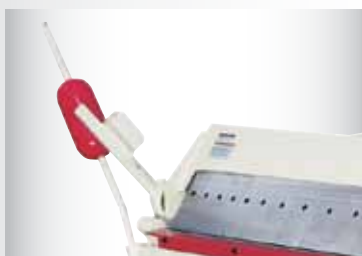
COUNTER WEIGHTS CAN BE MOVED UP OR DOWN TO PROVIDE MORE OR LESS LEVERAGE
