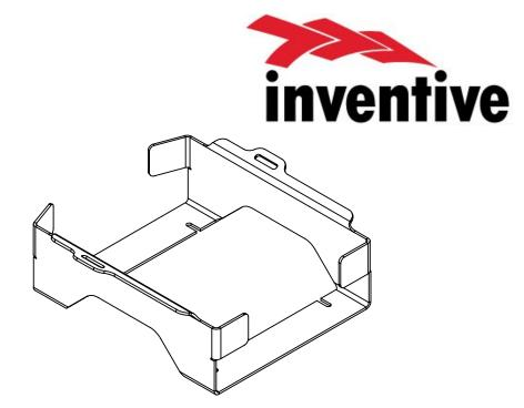
In The Ditch Towing Products PART NAME 5 gal Fuel Can Mount
