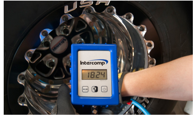
Intercomp's Digital Air Gauge provides racers the ability to make the precision air pressure adjustments that allow racing tires to perform at their best.
