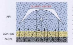
Narrow energy waves heat the **panel** not the air. With quartz infrared the **panel** is always warmer than the coating, and the coating is always warmer than the air above. Solvents and water are forced out quickly.
