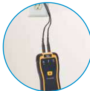
Traces on de-energized circuits
