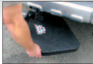
Rotate step underneath vehicle for travel
