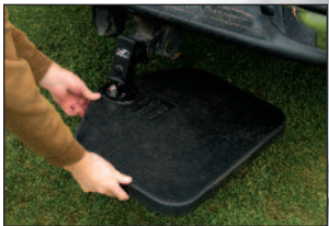
Rotate step underneath vehicle for travel
