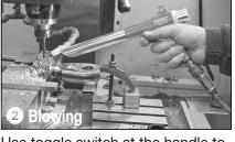
Use toggle switch at the handle to change between suction and blowing. Further conversion is not necessary.
