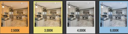
Correlated color temperature (CCT), an important aspect of LED lighting, characterizes how "cool" (bluish) or how "warm" (yellowish) nominally white light appears. CCT of a light source, given in Kelvin (K), defines the color tones of the emitted white light and is not an indicator of lamp heat. The chart below shows a range of CCT.
