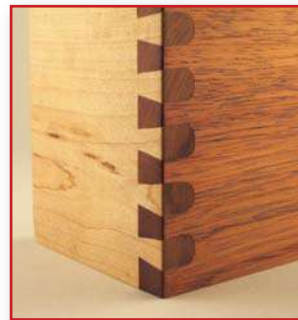
Cuts Through Joints
