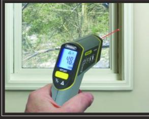
General Tools can help with the IRT207 Infrared Thermometer. Scan around windows in your home with the IRT207 to check for temperature variations. This can help determine if surrounding walls have gaps in
