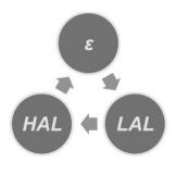
Also remember that when  $\epsilon$ , LAL or HAL is flashing, you have only 30 seconds to change its value or setting by pressing the  $\leftarrow$  LOG button or the °F/°C  $\rightarrow$  button. Thirty seconds after the last button push, the IRT659K's Auto Power Off function will activate and shut down the unit.
