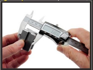
the calipers around the object in question in order to receive an accurate measurement.
