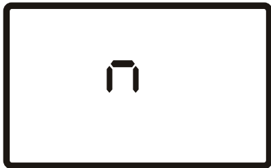
Fig. 10. The display indicating that the auto power off function has been disabled.
