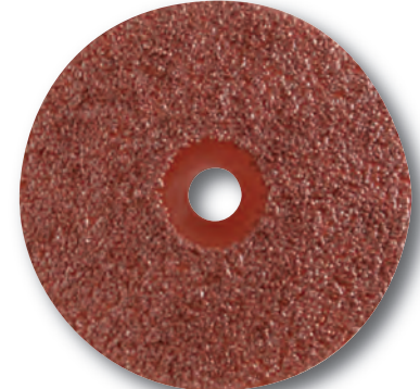
Zone Coated: Grain is placed, leaving a clear Zone around the arbor. Easier to lock on a grinder and provides a tighter fit. Excellent on coarse grits, where grain can be a hindrance.
