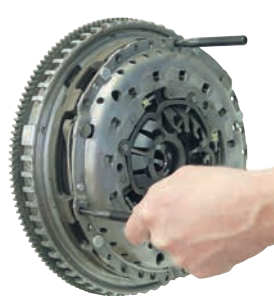
17. Remove knurled nuts, clutch pre-compressor and threaded bolts. Remove clutch aligner.
