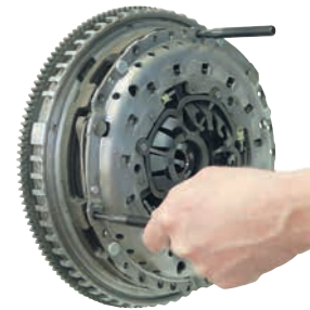
12. Remove knurled nuts, clutch pre-compressor and threaded bolts. Remove clutch pressure plate.
