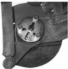
Pressing out the drive shaft flange
