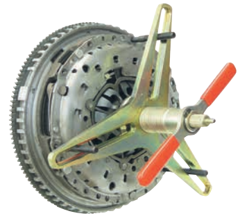
15. Screw down threaded bolts. Mount clutch pre-compressor.
