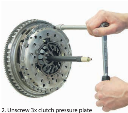
2. Unscrew 3x clutch pressure plate fastening screws. Replace with threaded bolts. Install clutch pre-compressor.
