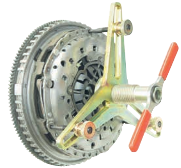
9. Compress diaphragm spring.
