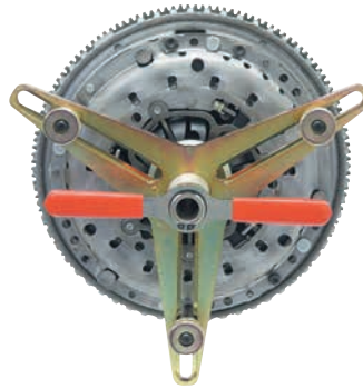
8. Screw in threaded bolts. Mount clutch pre-compressor.
