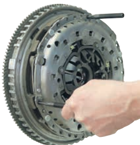
4. Remove knurled nuts and clutch pre-compressor. Remove clutch aligner and threaded bolts.
