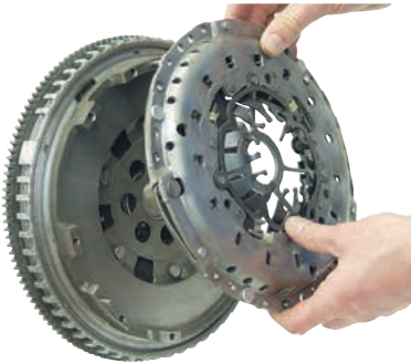
7. Install clutch pressure plate without clutch disc.
