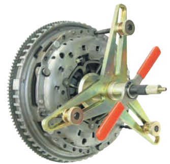
3. Compress diaphragm spring. Unscrew remaining fastening screws. Release pressure on diaphragm spring.
