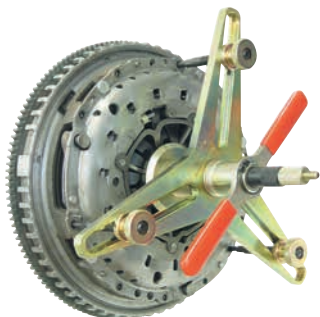
16. Compress diaphragm spring. Screw in fastening screws. Release pressure on diaphragm spring.
