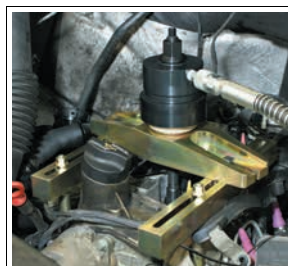
Extraction of injection nozzle in conjunction with KL-0583-10 K
