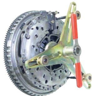
11. Release pressure on diaphragm spring. Remove reset tool.
