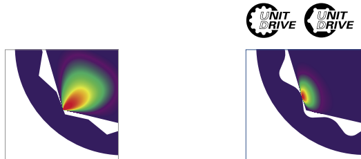
cold forged Fibers are bent and thus not as stable
