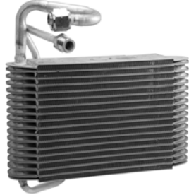
54590 Depth Height Width 2-7/8 13-5/8 7-5/8 Plate & Fin Evaporator Core O-Rings: (2) 24608 , (2) 24612 Buick (99-94); Olds (99-94); Pontiac (99-94)
