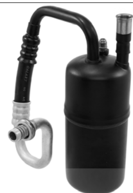
83042 Accumulator w/ Hose Outside Dia.: 3.500 Length: 9.000 Inlet Fitting Type: Female Springlock Outlet Fitting Type: Male Springlock Outlet Fitting: 5/8" O-Rings: (1) 24676 , (1) 24220 , (3) 24670 Ford (05-01); Mazda (06-01); Mercury (05) Ford: YL8Z19C836AA, YL8Z19C836AB Mazda: EC01615AOC
