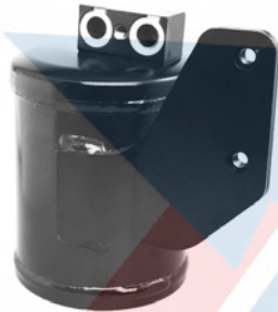
33995 Steel Filter Drier Outside Dia.: 4.000 Length: 6.250 Inlet Fitting Type: Pad Mount Outlet Fitting Type: Pad Mount
