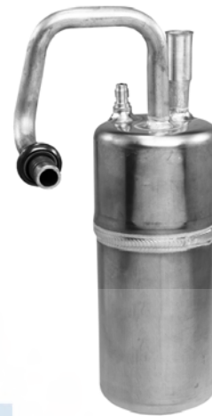
33155 Accumulator Outside Dia.: 3.500 Length: 12.000 Inlet Fitting Type: Male Springlock Inlet Fitting: 5/8" Outlet Fitting Type: Female Springlock Outlet Fitting: 5/8" O-Rings: (1) 24220 , (3) 24670 , (2) 24650 Ford (94-88); Mercury (94-88)
