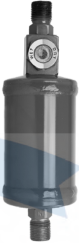
33992 Steel Filter Drier Outside Dia.: 2.500 Length: 8.250 Inlet Fitting Type: Male Insert O-Ring Inlet Fitting: 1/2" Outlet Fitting Type: Male Insert O-Ring Outlet Fitting: 1/2"
