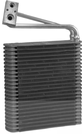
54568 Depth Height Width 3-1/8 16-3/8 4 Plate & Fin Evaporator Core Inlet: Block Fitting Outlet: Block Fitting O-Rings: (1) 24149 Chrysler (95-92); Dodge (95-91); Plymouth (95-91)
