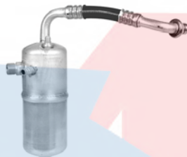
83013 Accumulator w/ Hose Outside Dia.: 3.500 Length: 9.500 Inlet Fitting Type: Male Springlock Outlet Fitting Type: Male Insert O-Ring Outlet Fitting: 5/8" O-Rings: (2) 24676 , (1) 24222 , (3) 24672 Ford (98-97) Ford: F75Z19C836AA Red Dot: 74R5077
