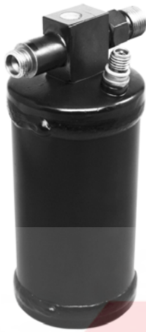
33986 Steel Filter Drier Outside Dia.: 2.500 Length: 6.500 Inlet Fitting Type: Male Insert O-Ring Inlet Fitting: 3/8" Outlet Fitting Type: Quick Disconnect Outlet Fitting: 1/4" Chevy (93); GMC (95-85)
