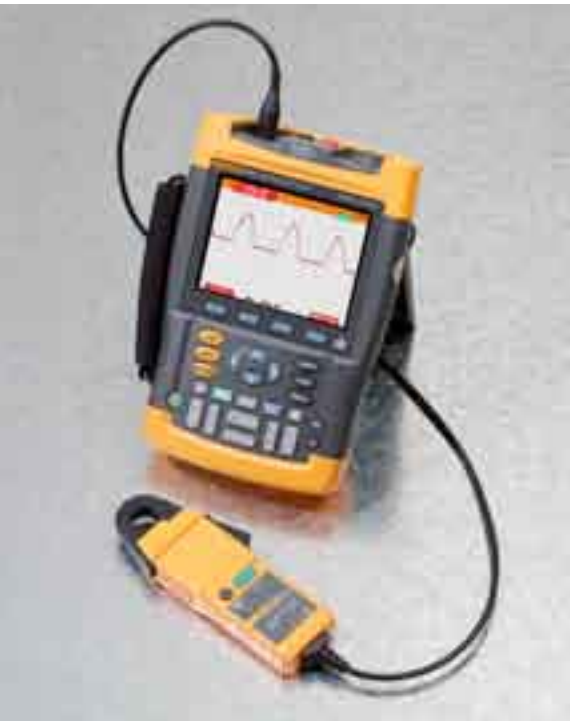
i30s connected to a Fluke 199C ScopeMeter.
